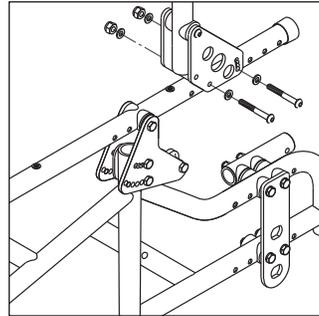
**Important Note:** This adjustment may also require re-positioning the seat-to-back bracket (underneath the solid seat) into the second set of mounting holes.
