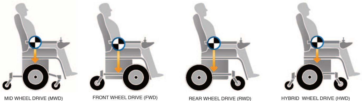
MWD has the client's center of gravity over the drive wheel. FWD has the client's center of gravity well behind the drive wheel. RWD positions the client's center of gravity ahead of the drive wheel. HWD Hybrid drive has the drive wheel position in between that of a mid and rear wheel drive.
