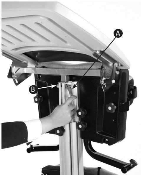
**!** Always use caution when making this adjustment, as fingers could become trapped in the slot while positioning.
