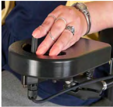
Switch-It MicroPilot uses pressure for activation
