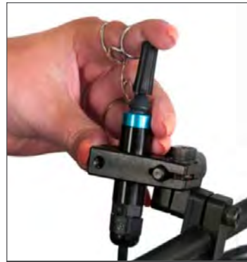
Switch-It MicroGuide uses joystick displacement for activation
